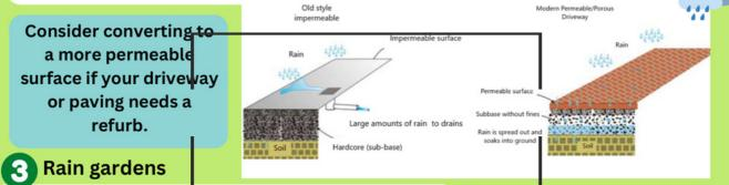
Rain gardens are a type of Sustainable Urban Drainage System (SuDS) which can be installed in your garden to help reduce flooding. Rain gardens store rainwater and release it slowly into the ground or sewer
